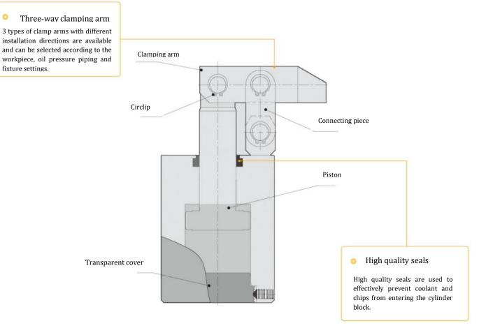
The figure shows the sectional view of the YGG-KB clamping state
