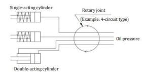
The hydraulic rotary joint effectively solves the problem that the oil pressure hose and fixed piping are difficult to supply oil to the rotary table of the machining center.
