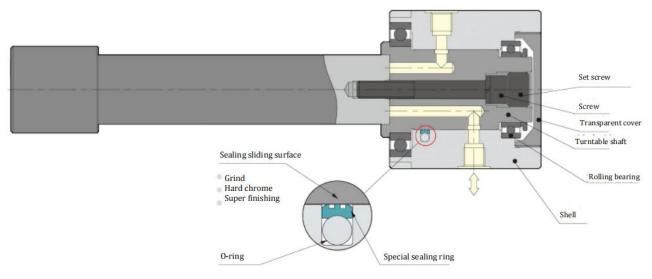
\*Disassembly method: unscrew the transparent cover, take out the set screw and M8 screw to separate the head and rod of the hydraulic rotary joint to disassemble it;
