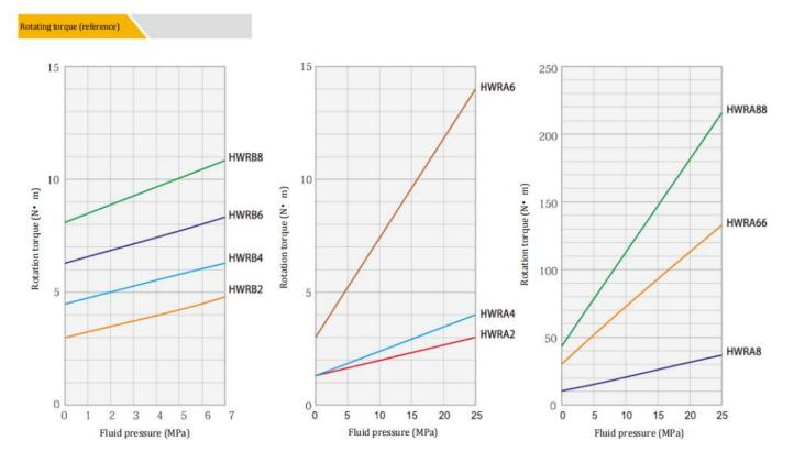
1. The figure above shows the torque during stable rotation (sliding resistance of the gasket).
