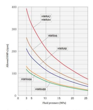
The pressure of the operating fluid, the rotation speed and the temperature of the operating environment interact, so they cannot be used at the maximum value at the same time.
