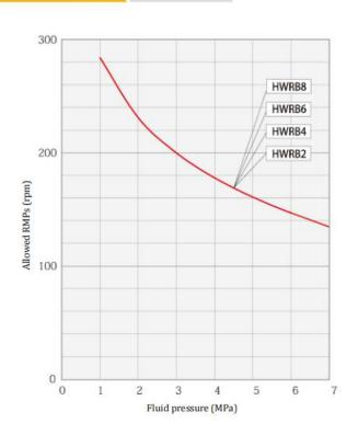
1. The figure above shows the allowed RMPs when a proper lubricating film is formed.
